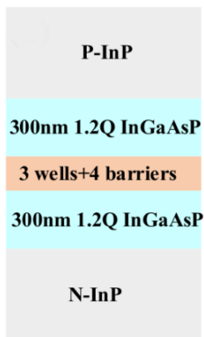
Figure: 1.5 \mu m InGaAsP laser schematic, adapted from Q. Ke et al.
